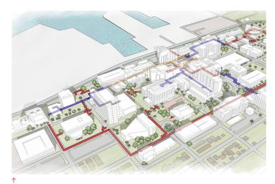
University of Texas Medical Branch at Galveston. Illustration of AEI design for resilience in campus infrastructure. After the devastation of Hurricane Ike (2008), the campus invested in combined heat and power plants, hot water distribution with building conversion and new energy and utility distribution/collection networks.
